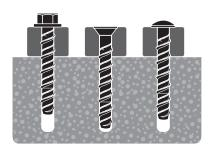
4 Continue to tighten the anchor until flanged head is firmly seated against fixture. Be sure not to over torque the anchor.
