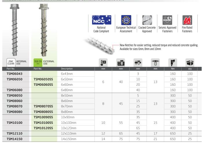
C1 Seismic assessment only valid for the following embedment depths: TSM06 - 40mm + 55mm / TSM08 - 65mm / TSM10 - 85mm / TSM12 - 100mm / TSM14 - 115mm. = Impact screwdriver maximum torque capacity, excessive torque during installation may damage the anchor. Training, expectise and good judgment is required.
