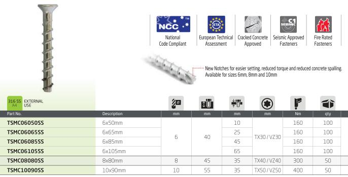
C1 Seismic assessment only valid for the following embedment depths: TSMC06 - 40mm + 55mm / TSMC08 - 65mm / TSMC10 - 85mm.
